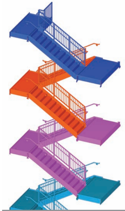
A screenshot of a BIM model of a McGregor Stair System created using Tekla. Tekla is used to detail all McGregor Stairs in house.
